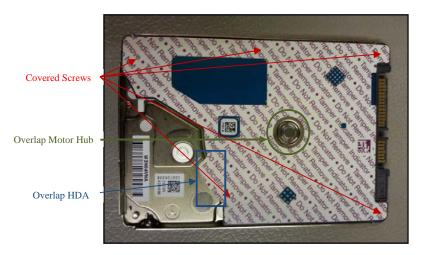
Security labels on top cover of drive to provide tamper-evidence of HDA cover removal
